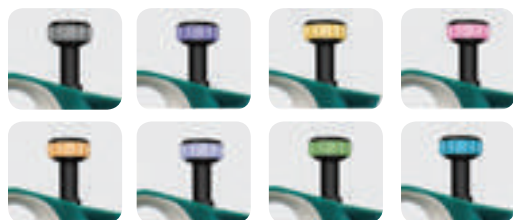
Color Coding: Different volume range micropipette dials are color-coded for easy identification.
